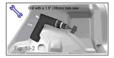
(e) Use a 1.5" (38 mm) hole saw to drill hole for the wiring harness. Make sure to drill all the way through the panel. (Fig. 10-2)
