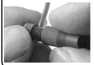
Make sure not to cross thread the cap when screwing it back in place.
