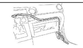
Make sure the end with the 6 pin Molex connectors is toward the radio. Run the BTAH harness behind radio, dash and along the edge of the vehicle until you get to the place you have decided to mount the tube.
