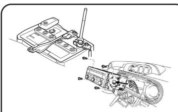
Disconnect negative battery clamp from battery. For easiest installation remove the radio and disconnect the harness from the back of the radio.
