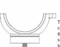
To use the center mounting configration, place the supplied 6mm hex head bolt in the counter sunk hex shaped hole. Use supplied locking nuts and washers to mount your accessories.
