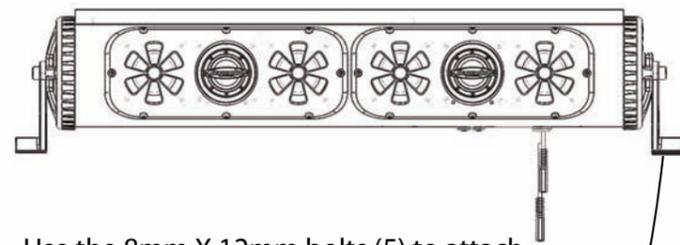
Use the 8mm X 12mm bolts (5) to attach the mounting legs. Mounting legs (3) can be installed in either direction depending on space constraints. When mounting with optional clamps (PR-URM, PR-FRC200, and PR-FRC175) use the hex bolts provided with the clamps to mount the bottom half of the clamps to the mounting legs.
