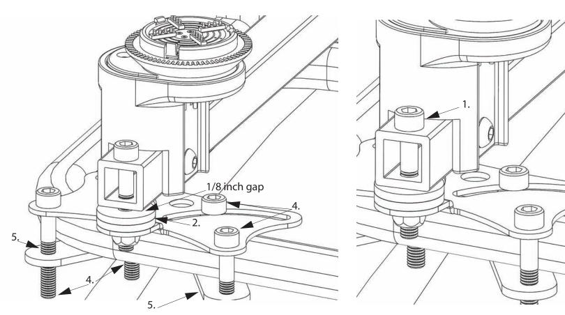
Screw 4 bolts (4) with washers into threaded mounting plates (5). Rotate bolts and mounting plates until bolts are against rack tubing. Then tighten all 4 bolts evenly. You will have a 1/8 inch gap between spacers (2) and mounting arm after mounting plate is tightened against the atv rack tubbing.
